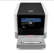
Place the assembled Chip, 10x Chip Holder and 10x Gasket in the tray and press the button on the touchscreen to retract the tray
