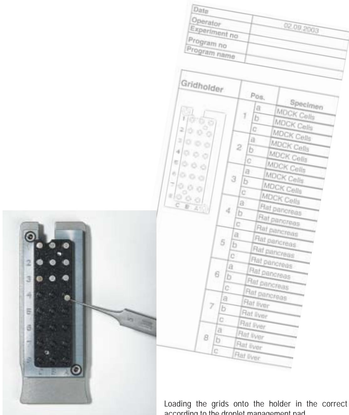
Loading the grids onto the holder in the correct position according to the droplet management pad.
