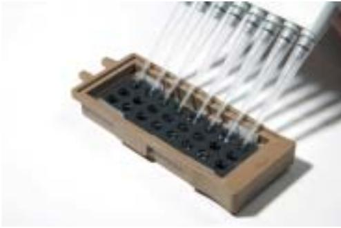
Using a multi 8-channel pipette for fast and accurate addition of wash and buffer droplets.
