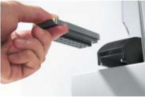
Loaded grid holder with grids facing down is placed into the grid station of the LEICA EM IGL.
